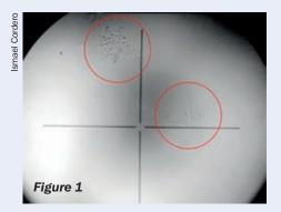
In its initial stages, fungus, as pictured in Figure 1, may not be perceivable by the clinician. However, over time the fungus will cover the lens surface in a web-like manner, initially causing a very slight loss of image brightness, followed by decreased contrast due to light reflecting off the fungus. In its final stages, the fungus etches the outer coatings of the lens and image sharpness deteriorates.
